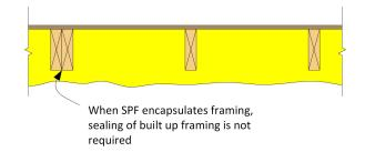
2. The SPF layer needs to completely encapsulate the interior UVA space so there are no gaps in the insulation or airtightness. In practical terms, this means that SPF must extend down and connect to the air barrier for above-grade walls such that discontinuities do not exist at eaves and projecting roof assemblies. (See Figure 3.2)
