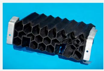
Plastic honeycomb floor rocker reinforcement
