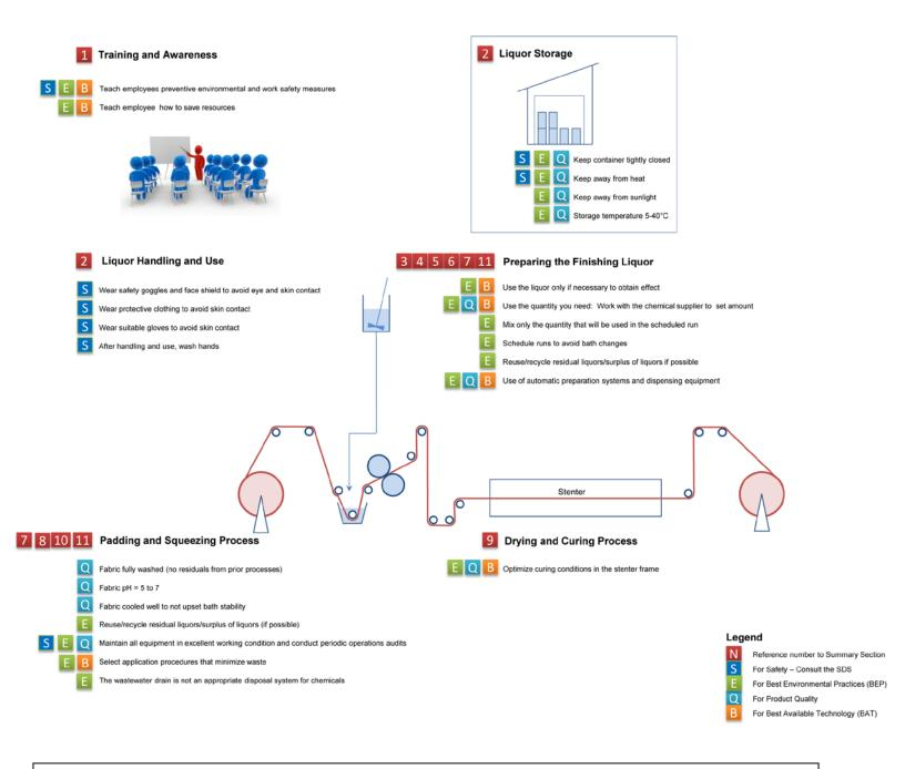
**Figure 1:** Overview of Best Environmental Practices (BEP) when using fluorinated repellent products in the textile industry (numbers refer to summary section on page 1).
